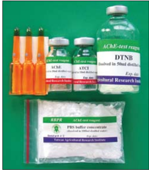
Fig. 14. The kit for pesticide detection of AChE
