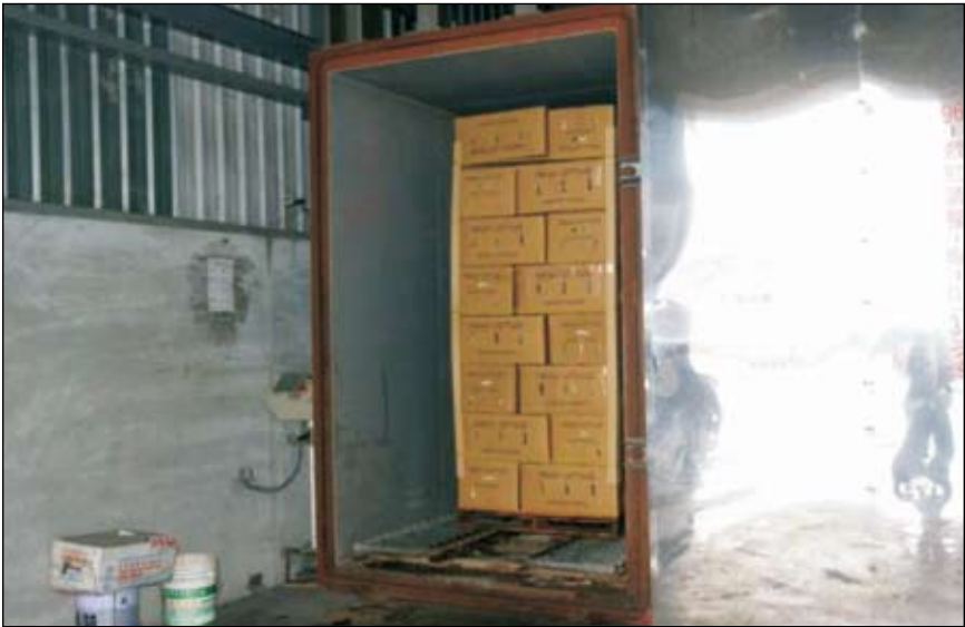
Fig. 23. Head lettuce under finishing vacuum cooling treatment
