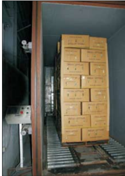
Fig. 22. Head lettuce before vacuum cooling treatment
