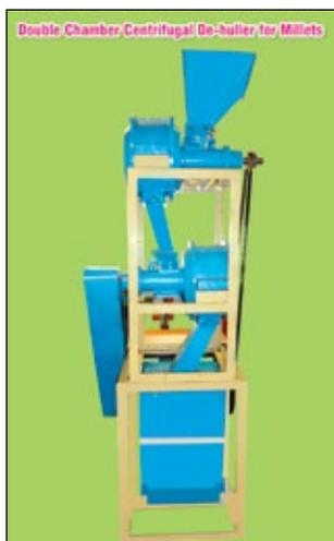
The characteristic features of the variety are : i) 10 per cent more recovery (since the bran is retained in the kernel); ii) suitable for little millet, proso millet, foxtail millet, barnyard millet and kodo millet; iii) the capacity of the de-huller is 300 kg per hour; iv) the efficiency of the unit is 95 per cent; v) breakage of 4-5 per cent; vi) labour required: one person; vii) cost of the unit Rs. 1,20,000 (USD 1,758.75); and viii) cost of operation Rs. 5 (USD 0.07) per/kg.
