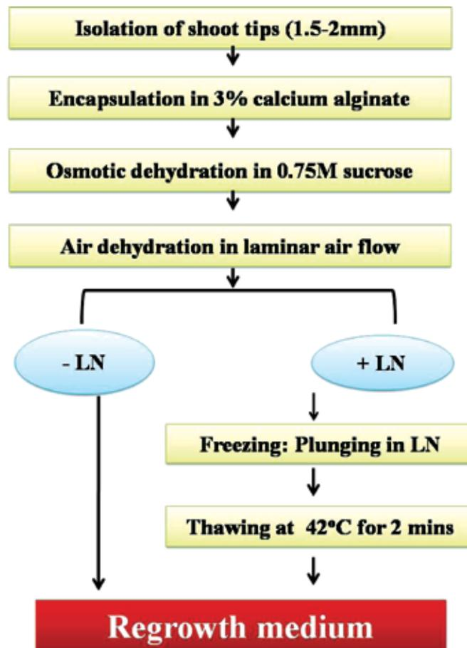
**Fig. 1:** Generic protocol for cryopreservation of shoot tips by encapsulation – dehydration technique
