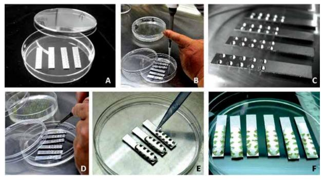
Fig. 1. Adhesion of shoot tips on the cryo-plates
