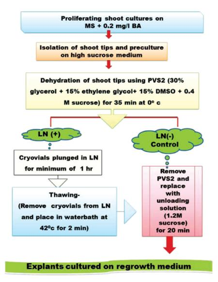
Fig. 2. Flow chart of cryopreservation of Bacopa monnieri using vitrification
