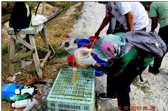
Figure 23: Measuring of ISR inoculant using measuring cylinder
