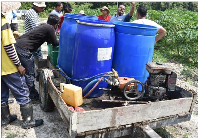
Figure 27: Complete set-up of four barrels, engine, pump, hose and AVLG
