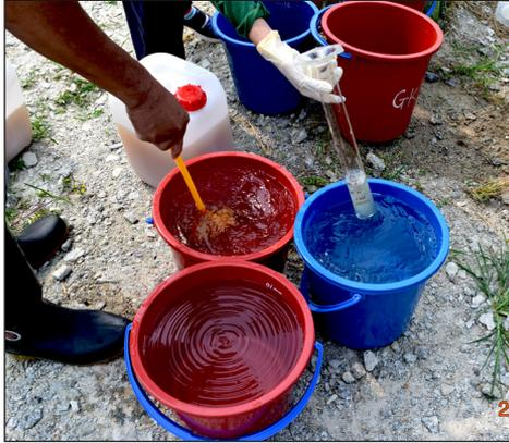
Figure 24: Dilution of ISR inoculant into pail containing 10 litres of water
