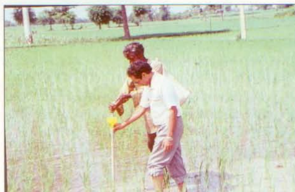
Testing Urea Super Granules (USG) in paddy fields, using indigenously fabricated USG Applicator; which leads to a saving of 20% fertilizer-nitrogen
