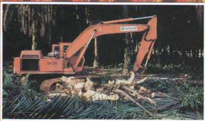
Excavator Fitted with Blade for Shredding Oil Palm Trees
