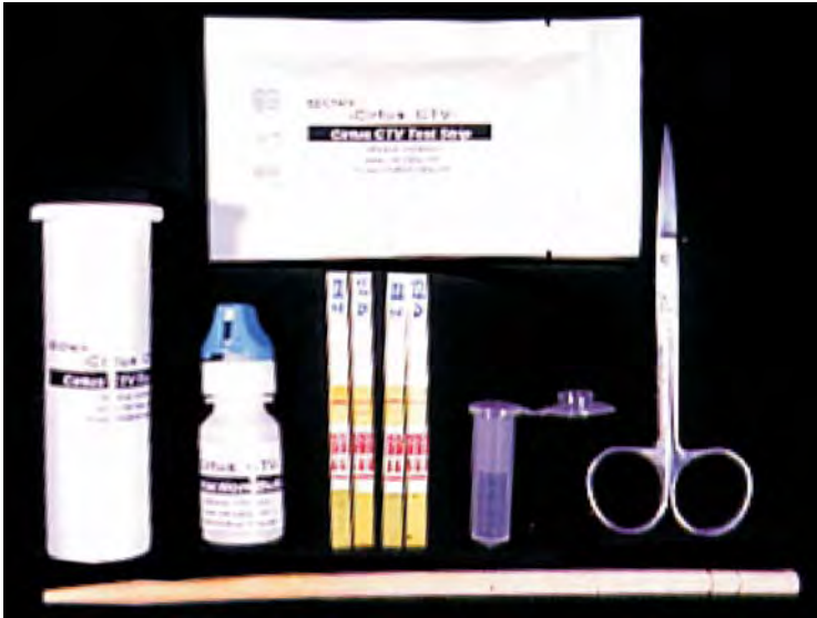
Fig. 19. Diagnosis strips for CTV detection, produced by Meikang Biological Project Co., Taiwan in collaboration with Plant Virology Laboratory, NTU.
